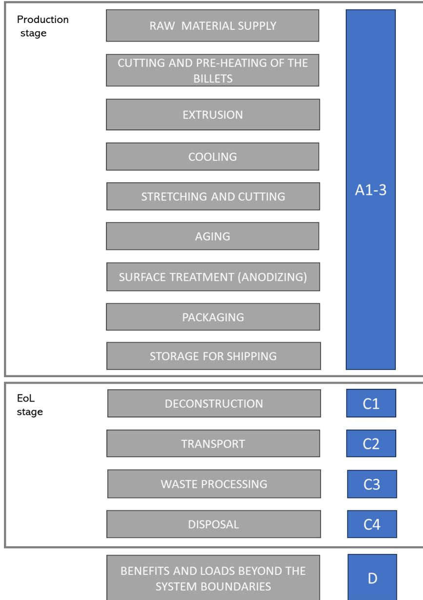
Figure 1: Scheme of the profiles manufacturing process occurring in Mountain Top
