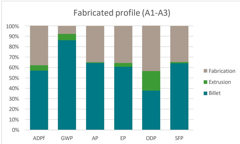
Figure 3 Relative contribution of upstream processes for fabricated profile
