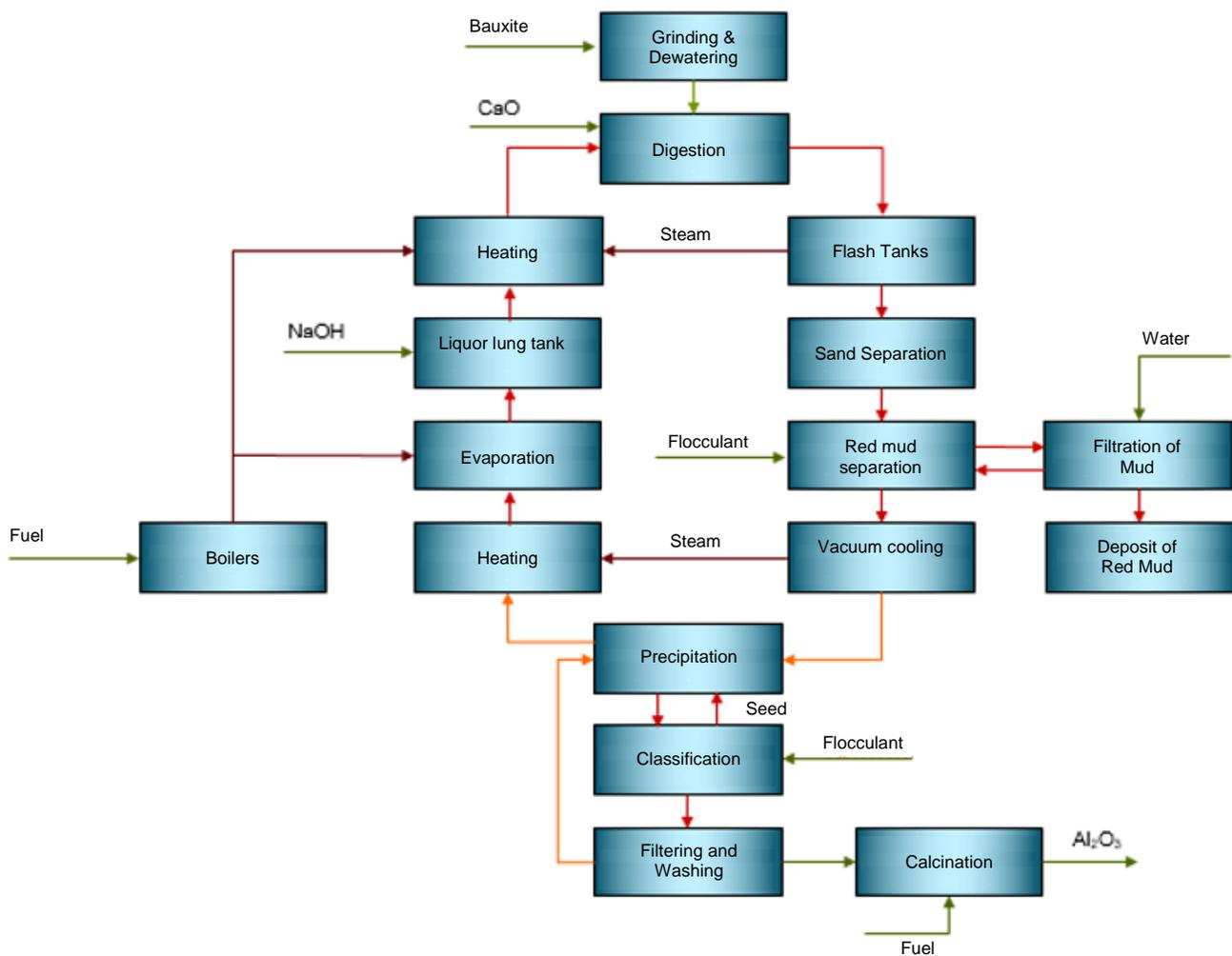
Figure 8 - Simplified Flowchart of the Bayer Process.
