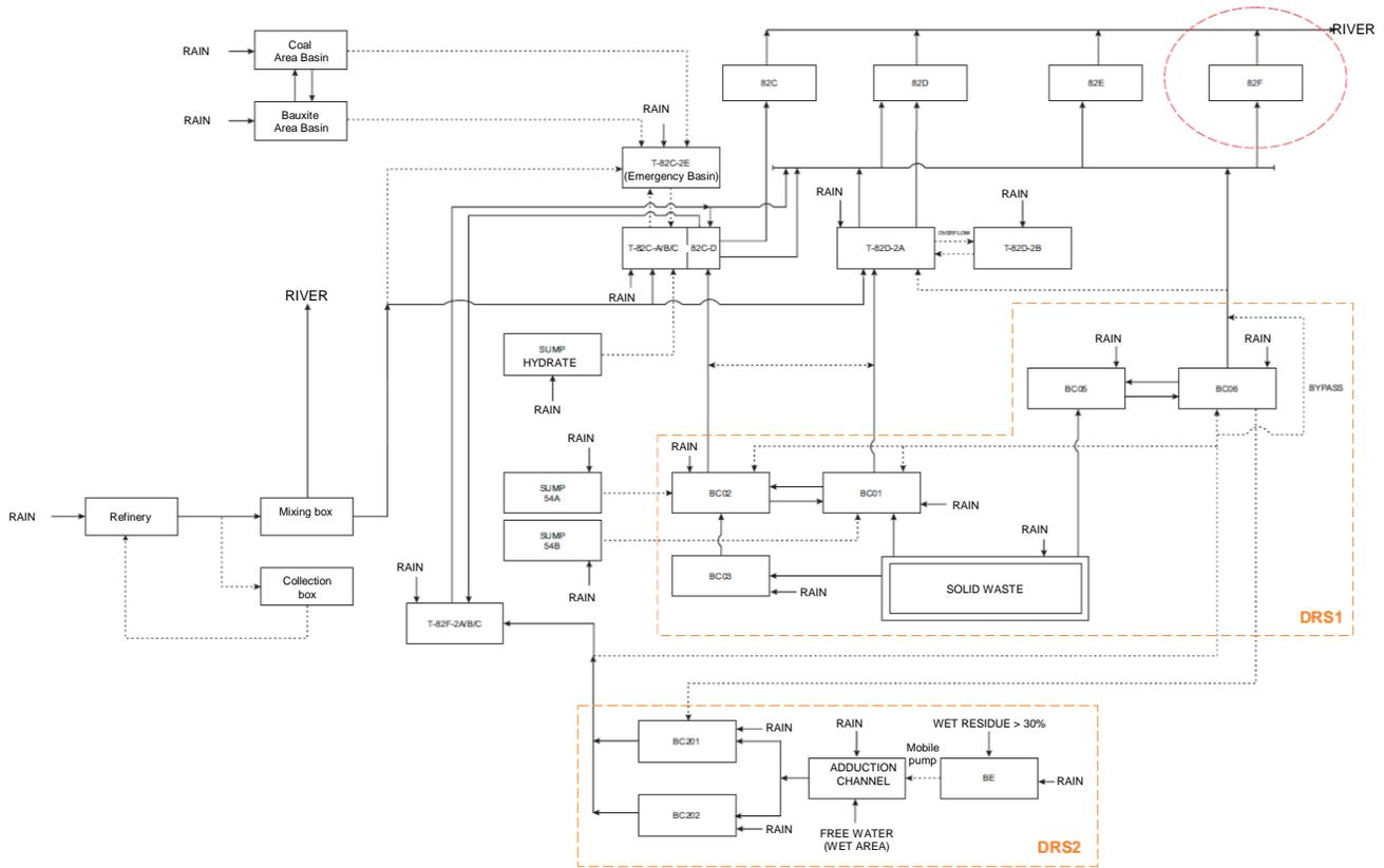
Figure 18 – PFD wastewater circuit in May 2019.
