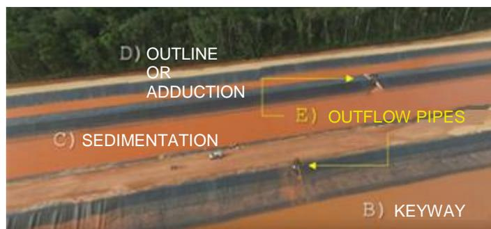
Figure 5 - DRS2 details showing overflow between channels.
