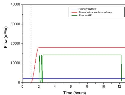
Figure 39 - Outflow generated by the refinery and the rain of 22.77 mm/h for 12 hours.
