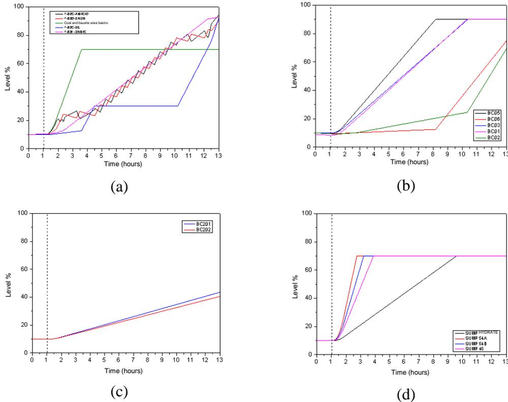
Figure 40 - Basins' level considering a rainfall of 22.77 mm/h for 12 hours, new catchment area, new pumping capacity and the PFD of December 2018.
