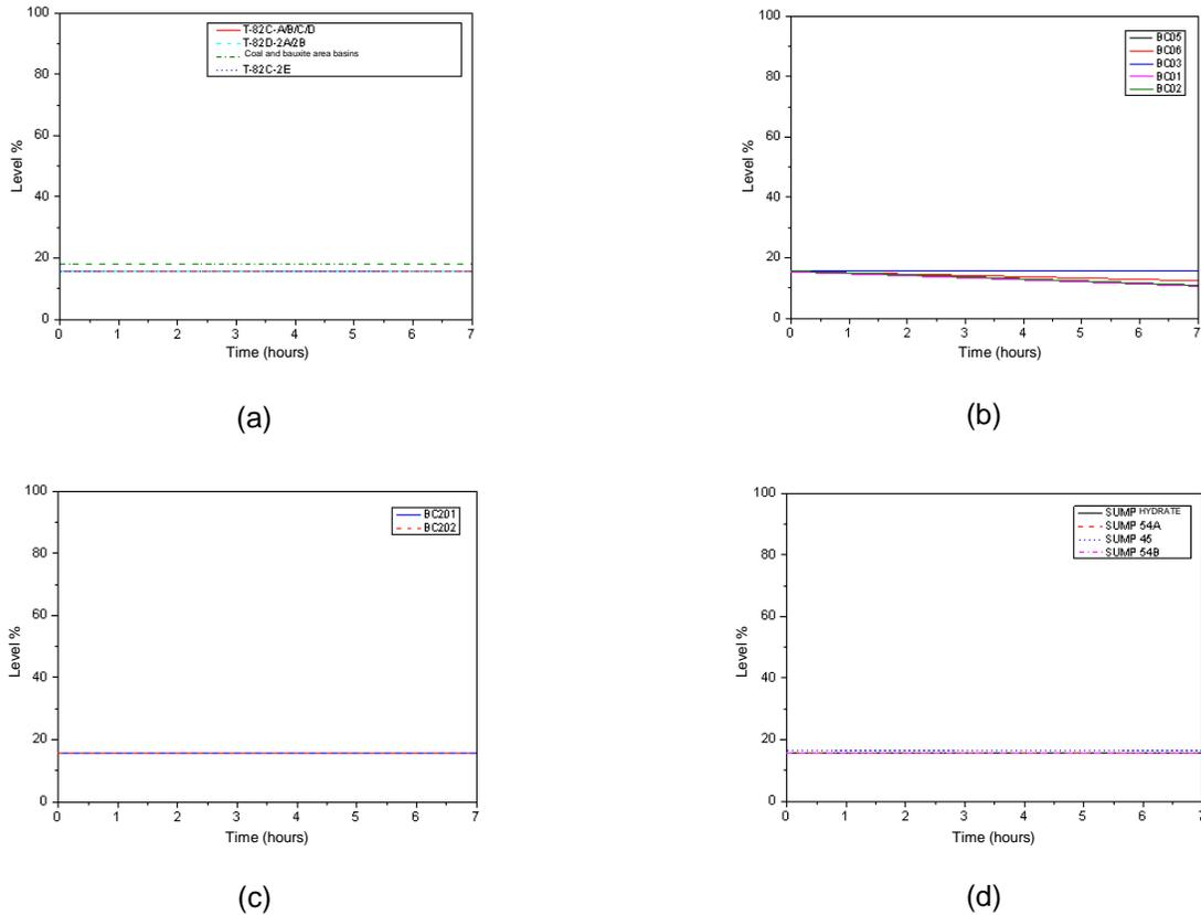
Figure 35 - Level of the basins and sumps for the increase in outflow, considering the PFD of February 2018.
