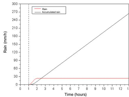
Figure 38 - Rain profile of 22.77 mm/h for 12 hours and accumulated water.
