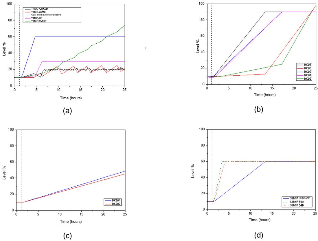
Figure 43 - Basins' level considering a rainfall of 12.86 mm/h for 24 hours, new catchment area, new pumping capacity and the PFD of May 2019.
