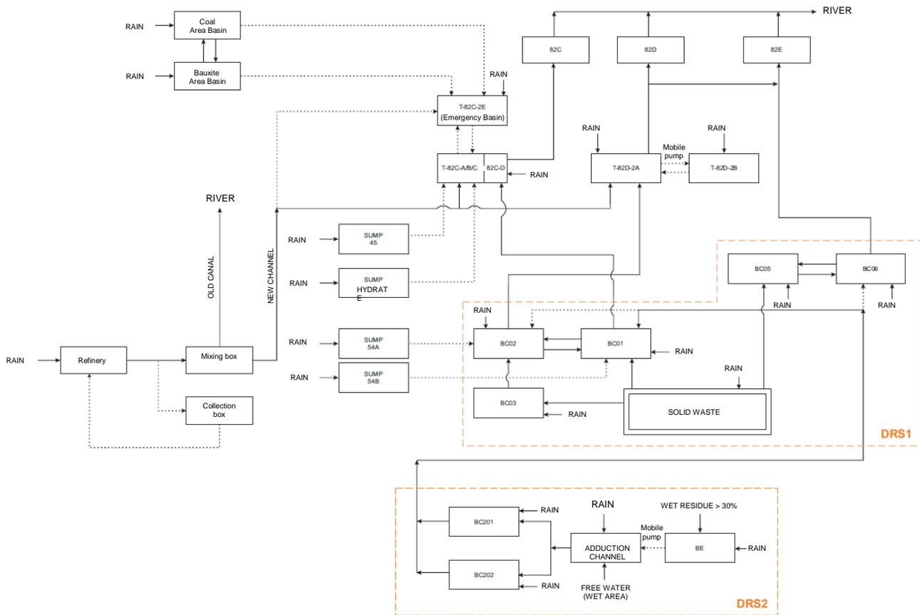
Figure 16 – PFD wastewater circuit in February 2018.
