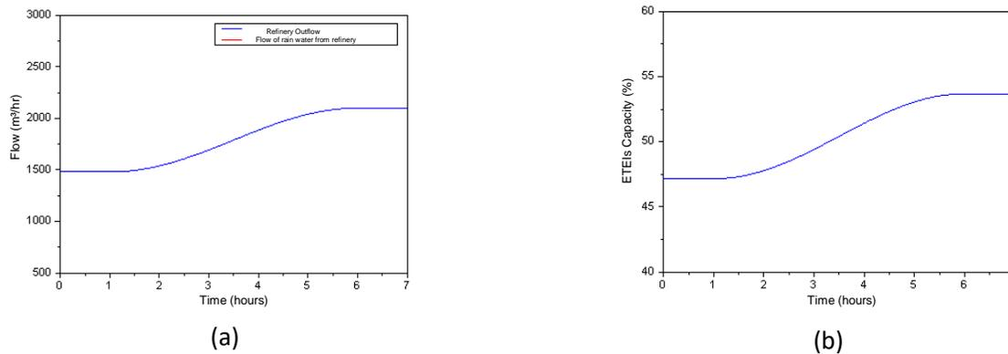
Figure 36 - Outflow and rainwater flow and percentage of use of ETEI, considering the PFD of February 2018.
