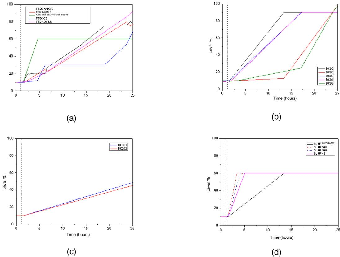
Figure 41 - Basins' level considering a rainfall of 12.86 mm/h for 24 hours, new catchment area, new pumping capacity and the PFD of December 2018.
