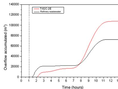
Figure 32 - Water accumulated inside Alunorte during the event of February 16 and 17, 2018, considering the PFD of February 2018.
