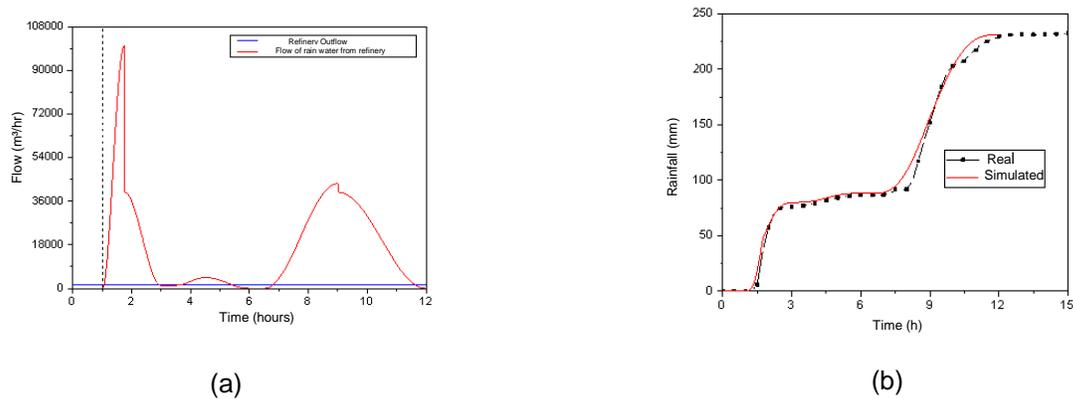
Figure 33 - Outflow from the refinery, water flow generated by rain during the event of February 16 and 17, 2018 and validation of the rain profile, considering the PFD of February 2018.
